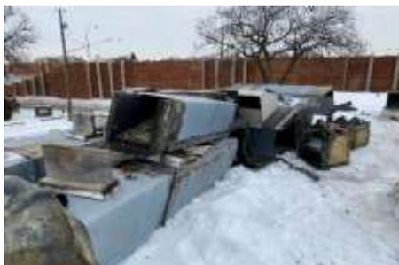
*Previous metal duct lined with fiberglass, severely damaged due to pooling water and harsh weather conditions over time.*
