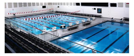
Natatoriums are challenging applications to deliver fresh air to the breathing zones of swimmers, people on the pool deck, and spectators. They are often highly humid spaces that can contain chloramine gas, a corrosive byproduct of pool chlorination, that hangs in the air and causes serious respiratory irritation.
